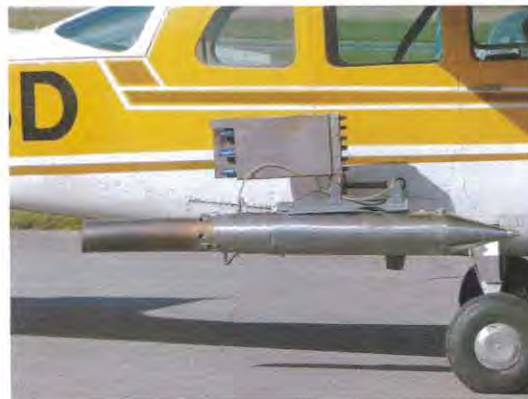
Cessna 210 with a device for cloud seeding with silver iodide.
